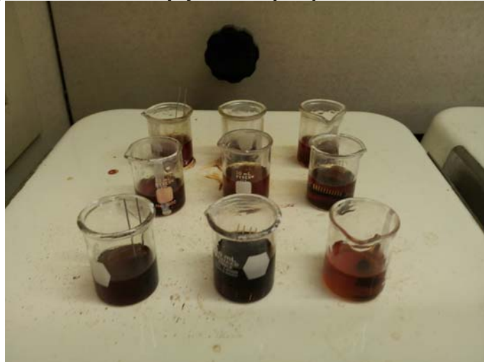
Figure 3. Solvent C (Dynasolve) Exposure at 45 minutes
