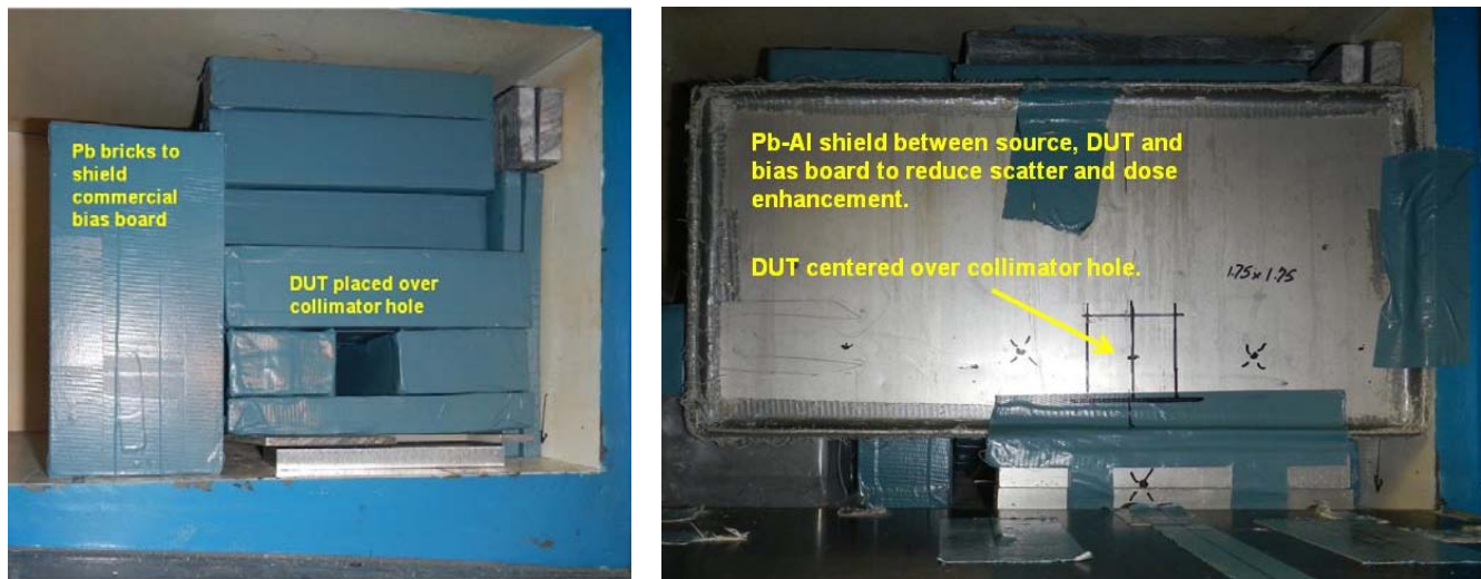
Fig. 3. Physical configuration of bias board shielding and DUT placement.
