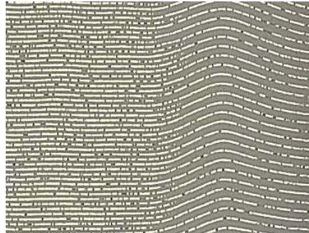
Figure 2 Acceptable undulation in electrode/dielectric layers
