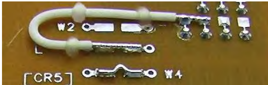
Figure 9-2. Single Wire Staking
