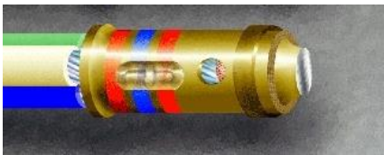
Figure 19-24. Contact Trimmed and Deburred
