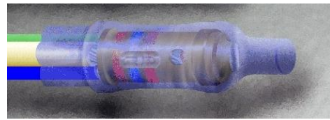
Figure 19-25. Contact Covered With Shrink Sleeving
