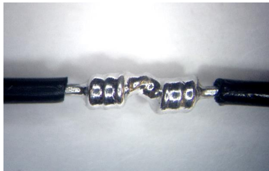
Figure 19-18. Soldered Western Union/Lineman Splice
