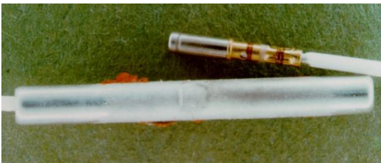
Figure 19-32. Crimped Contact Outside Junction Device
