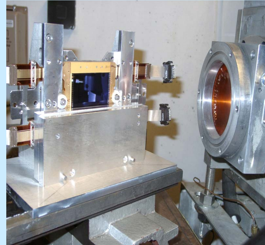
Hubble Space Telescope Wide Field Camera 3 EZV 2k x 4k n-CCD in front of Proton Beam at UC Davis Crocker Nuclear Lab (CNL). Photo by Paul Marshall, consultant to NASA
