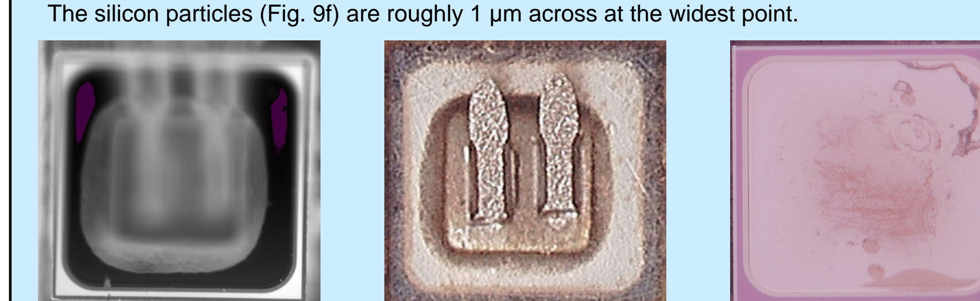
Fig. 9a. Thermal image of the irradiated SN2 does not identify any failure locations. Fig. 9b. No failure location is visible in the low-magnification optical image of the DUT. Fig. 9c. These discolorations are observed in the silicon of SN2 after the Schottky barrier metal, bond pad, and bond wires were removed.
