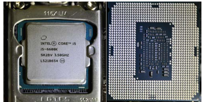
Fig. 1. Skylake i5-6600K Desktop Processor, socketed, revealing the topside markings (left) and un-socketed, underside view, (right).
