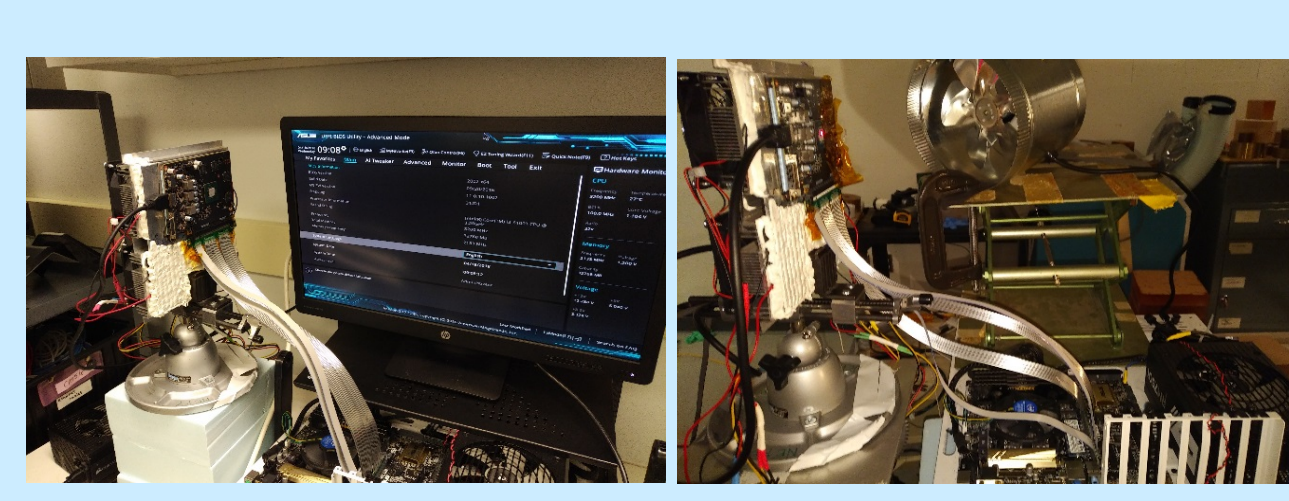
Figure 4: Reverse Side Modifications 400W Cooling on Bare NVIDIA GTX 1050
