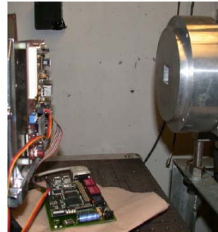
Figure 4: Virtex-4 Board in beam path.
