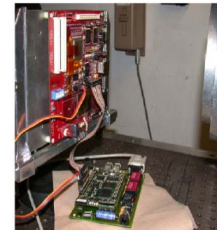
Figure 5: DSP/Virtex-2 board set away from beam.
