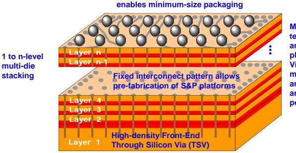
Multi-function, multitechnology, multiarchitecture S&P platforms – ViArrays, memories, 3D multi-core processor architecture, precision analog, HBTs, MEMS, power devices...
