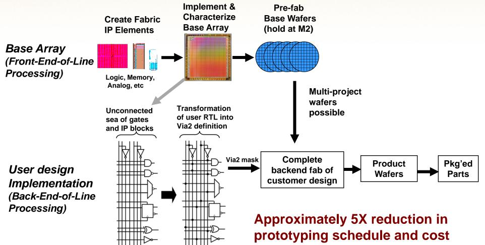
prototyping schedule and cos compared to cell-based ASIC approach
