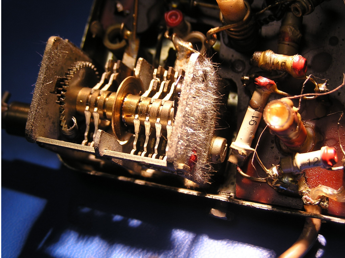
Tin whiskers from a 1960s era variable air capacitor (Courtesy of NASA GSFC)
