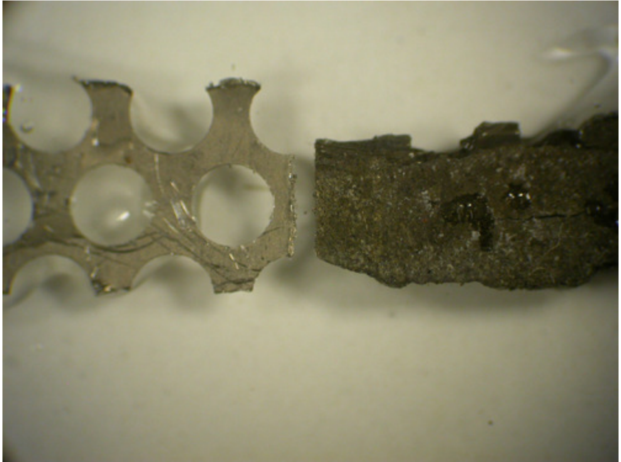
Harvested electrodes from a nickel cadmium cell, secured to a glass slide with epoxy
