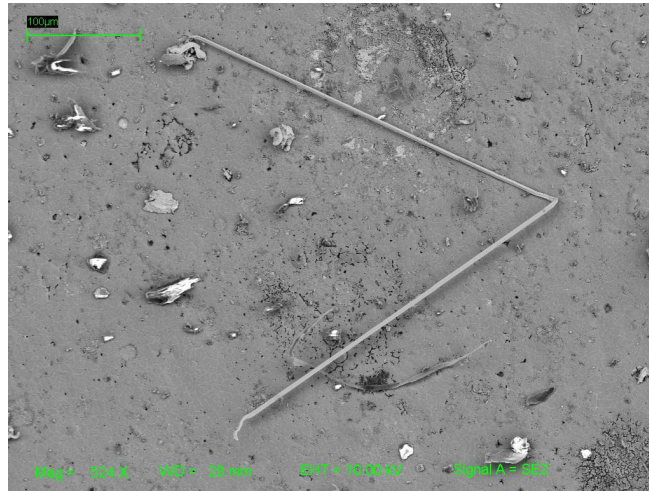
Scanning electron microscope image of a Cd whisker in battery switch (Courtesy of NASA GSFC)
