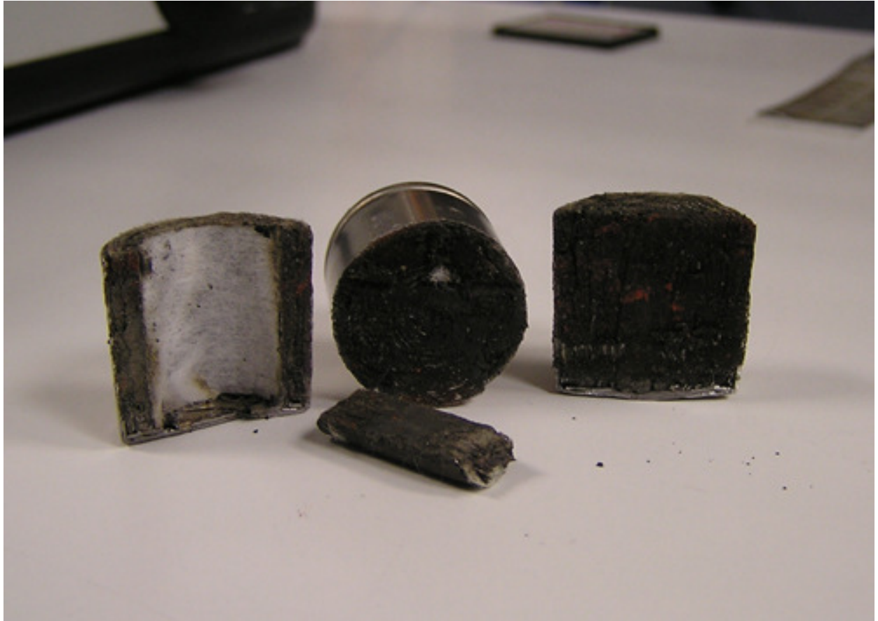
Disassembled Sanyo Cadnica nickel cadmium cell
