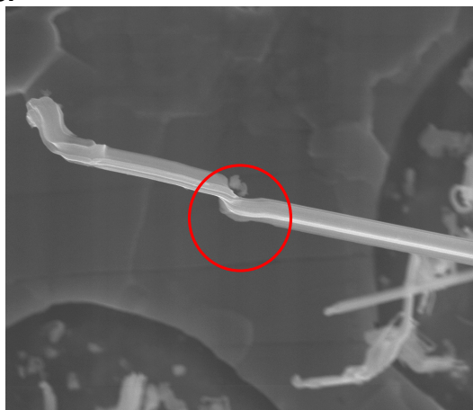
Storage at room temperature in air for 820hr, on the surface of CeSn 3 phase
