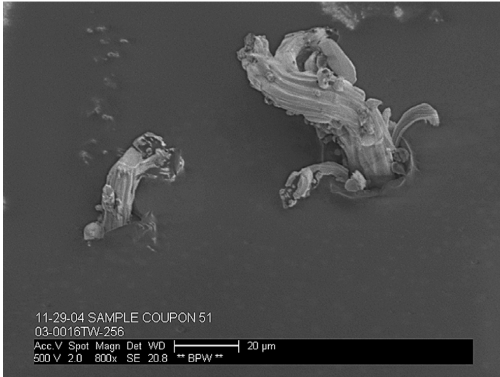
Figure 27. Whiskers Penetrating Coating D – 1.2 Mils (401 Days at Ambient + 347 Days in 25°C/97%RH)
