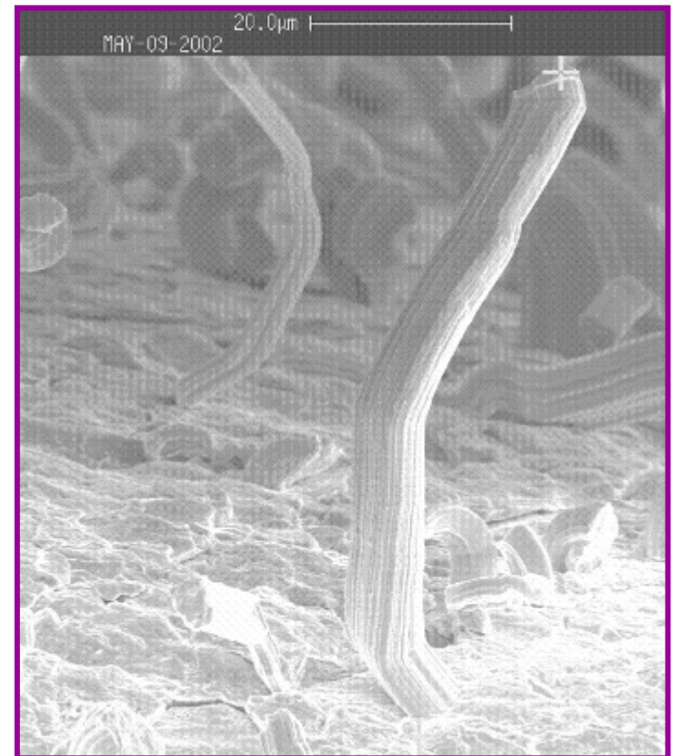
Tin Whiskers on Tin-Plated Ceramic Chip Capacitor
