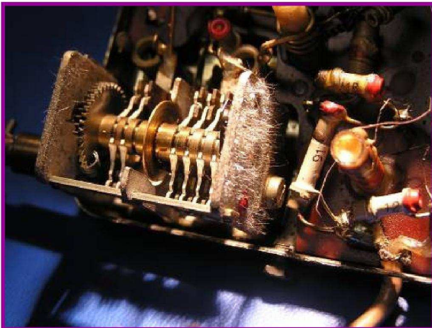
Fig. 1: Tin Whiskers on 1960s-Era Variable Air Capacitor [5]. Reproduced with permission from NASA
