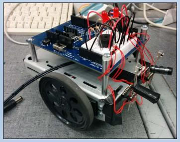
This robotic shield performs a set of programmed instructions utilizing two servo-controlled wheels, a piezoelectric element, IR LEDs and photo resistors.
