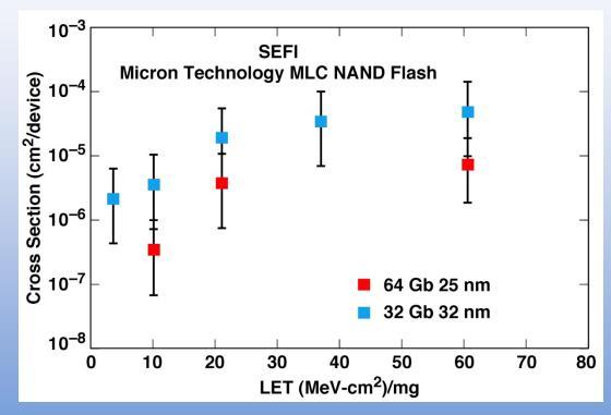
Scaling effect of SEFI cross-section for Micron MLC NAND flash memories
