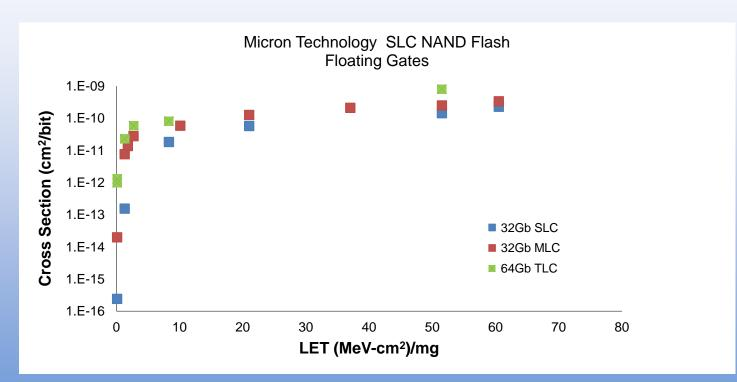
Comparison of SEU cross-section for Micron SLC, MLC and TLC NAND flash memories. Error bars are smaller than the plotting symbols.
