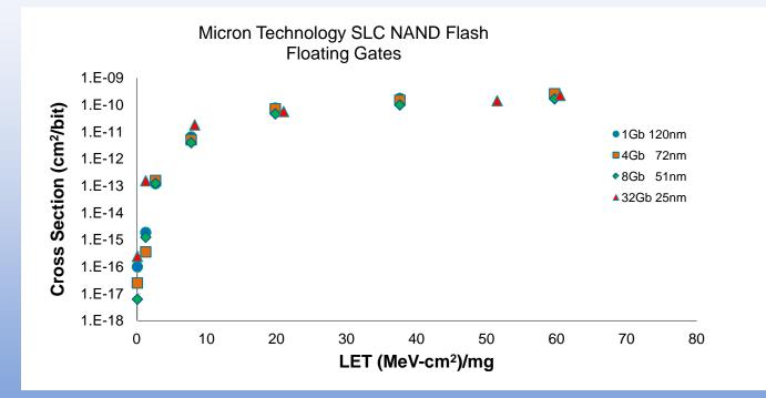
Scaling effect of FG SEU cross-sections for Micron SLC NAND flash memories. Error bars are smaller than the plotting symbols
