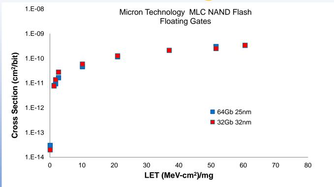
Scaling effect of FG SEU cross-section for Micron MLC NAND flash memories. Error bars are smaller than the plotting symbols
