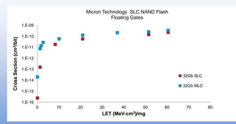
Comparison of SEU cross-section for Micron 32Gb SLC and MLC NAND flash memories. Error bars are smaller than the plotting symbols.
