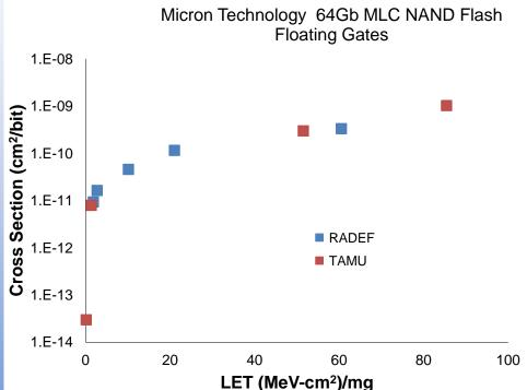
SEU cross-section for Micron Technology 64Gb MLC NAND flash memory. Error bars are smaller than the plotting symbols
