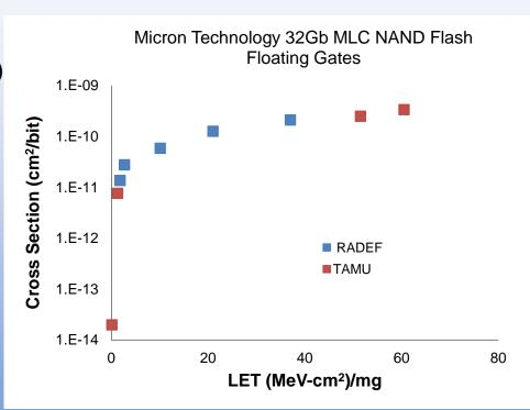
SEU cross-section for Micron 32Gb MLC NAND flash memory. Error bars are smaller than the plotting symbols
