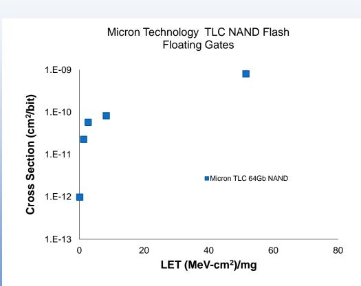
FG SEU cross-section for Micron 64Gb TLC NAND flash memory. Error bars are smaller than the plotting symbols.
