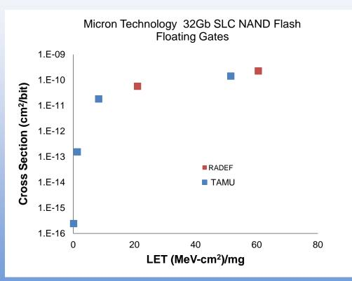
SEU cross-section for Micron 32Gb SLC NAND. Error bars are smaller than the plotting symbols
