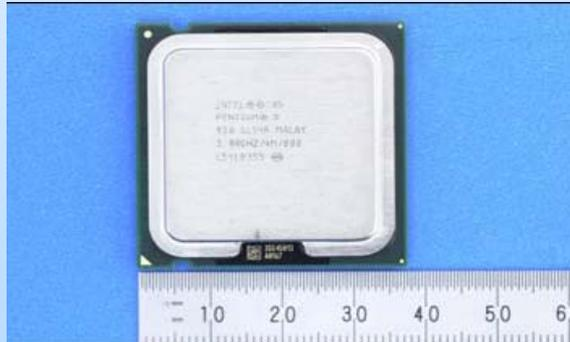
Intel 65nm Dual Core Pentium D Processor
