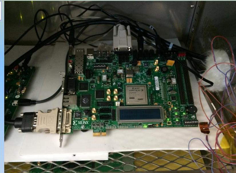
**Board mounted in the thermal Chamber During the Tests**
