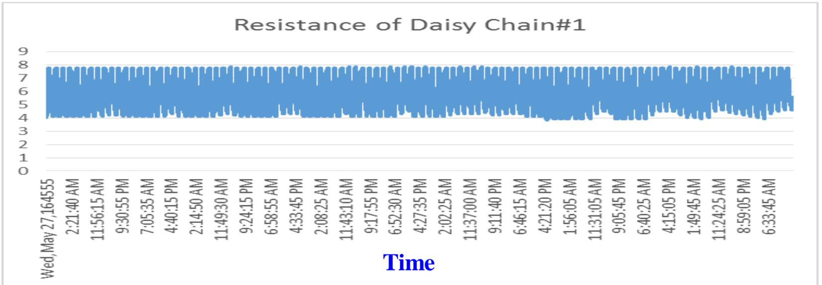
No change in daisy-chain resistance was observed which indicates no anomalies/failures.
