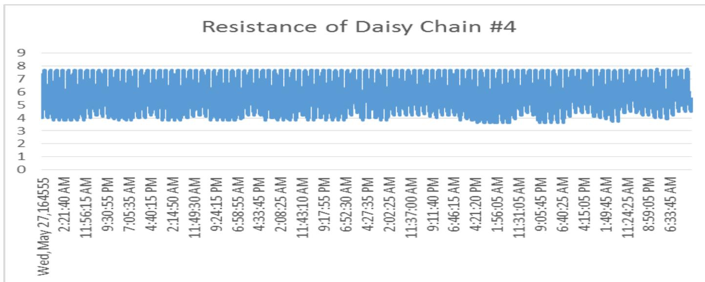
No change in daisy-chain resistance observed which indicates no anomalies/failures.
