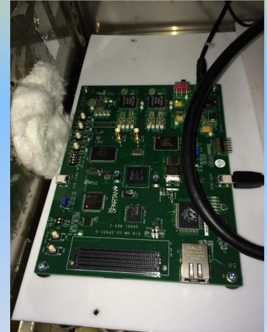
**Board mounted in the thermal Chamber During the Tests**
