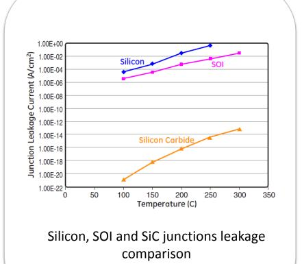
300°C SiC-based Analog and Digital Circuits
