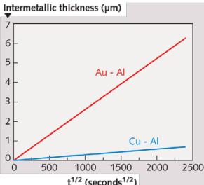
Comparison of Cu-AL and Au-Al IMC growth rate at 175°C. Figure taken from *Copper Wire Bond Failure Mechanisms* (Schueller, DfR Solutions) and recreated from Copper vs. Gold Ball Bonding (Breach)
