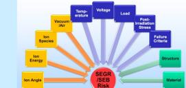
Parameters going into a SEE test on power MOSFETs
