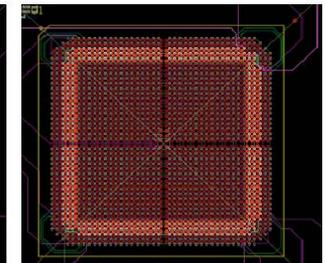
Figure 37: Daisy chain periphery (1 chain)
