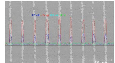
Figure 26: Elemental analysis of PME capacitor
