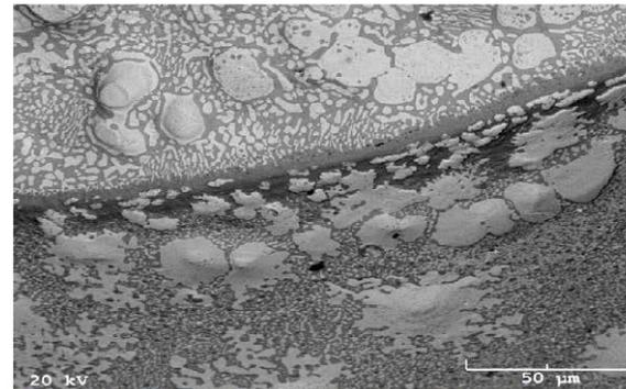
Figure 16: SnPb phase on the top of the column
