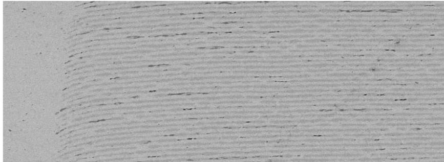
Figure 19: X-section of AVX BME capacitor
