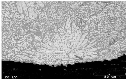
Figure 15: SnPb phases on the base of the columns
