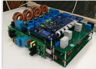
FSU Gen-I SiC PV converter prototype (~2.5 kW/kg)
