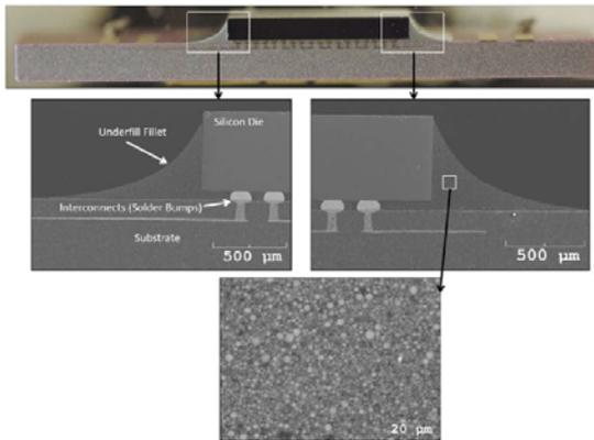
Cross section of a flip-chip die (top) with underfill fillet keyed to two diagrams (middle) showing the location and general arrangement of underfill around the chip components. Right diagram shows relationship to enlarged view of fillet (bottom) at 20 μm. (Photographs and micrographs were generated by R. Ruiz.)
