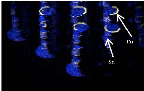
Figure 13: EDX image for the presence of Sn and Cu
