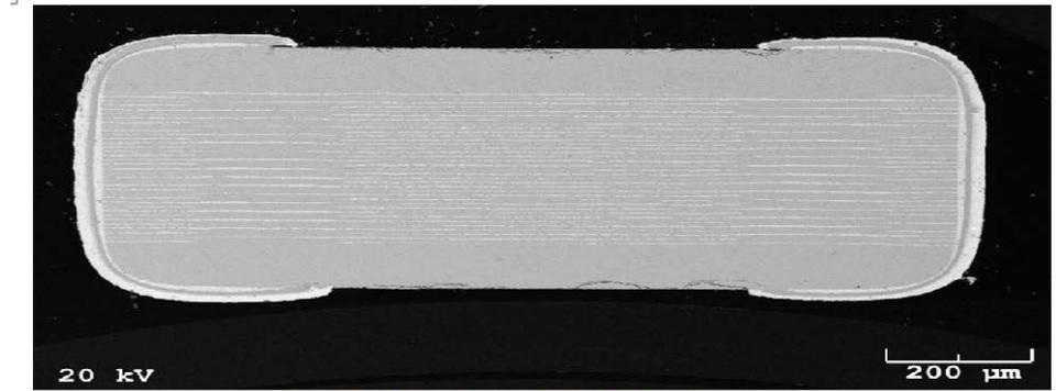
Figure 24: SEM image of PME capacitor from Presidio
