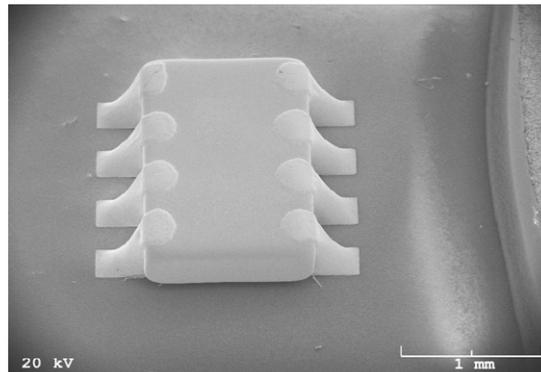
Figure 18: SEM image of capacitor
