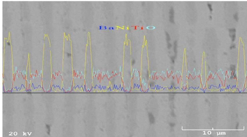
Figure 20: Elemental analysis of capacitor body
