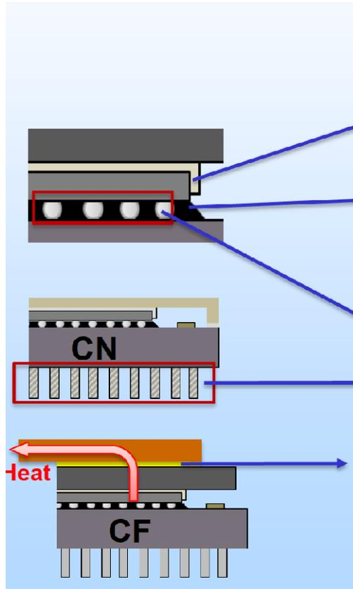
The diagram shows three cross-sectional views of CGA packages. The top view shows a chip on a carrier with a TIM1 layer and underfill. The middle view shows a carrier (CN) with six columns. The bottom view shows a carrier (CF) with a TIM2 layer and heat transfer device. Red arrows point from the diagram to the corresponding rows in the table.
