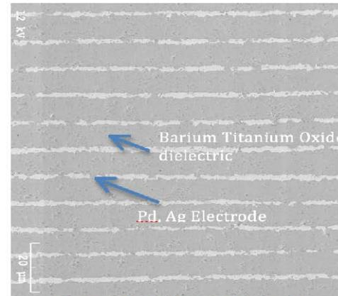
Figure 25: SEM image of PME Capacitor
