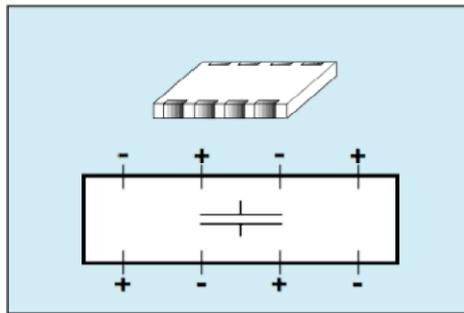
Figure 17: Schematic of AVX BME interdigitated capacitor (IDC)
