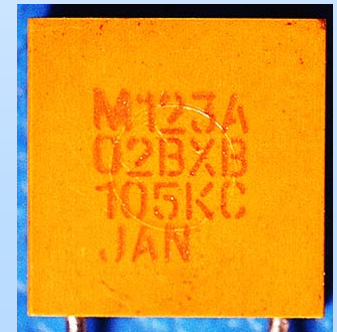
Ceramic Capacitor NASA GSFC PA Lab J14094
