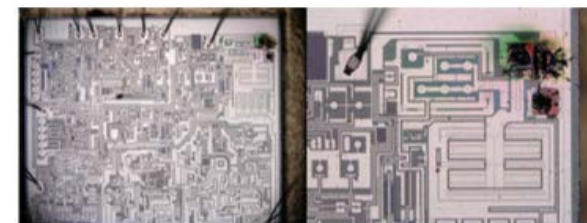
Fig. 7 Photomicrographs of a RH3845 that exhibited destructive SEE.
