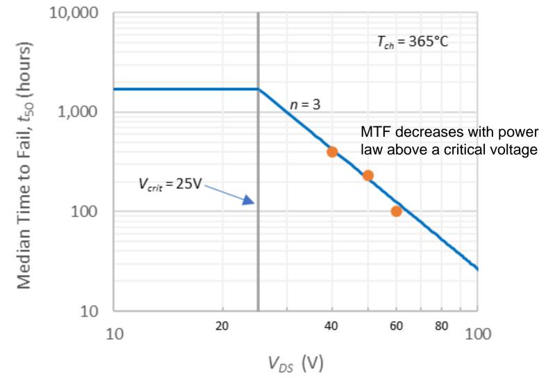
Not all HEMTs exhibit a voltage dependence of accelerated failure time
