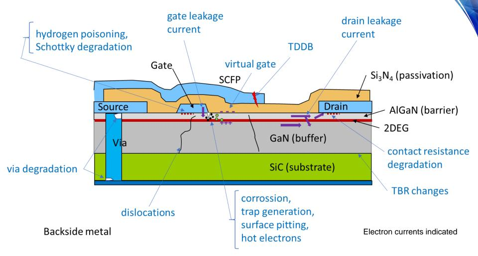
Different failure modes operate in different electrical regimes
