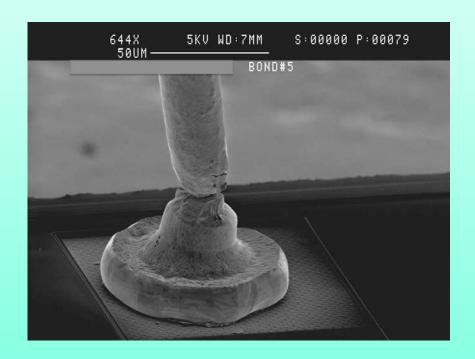
These unique deformations were caught due to a single failure at Bond Pull in a standard DPA of a Hermetic Microcircuit. Turns out to affect multiple lots. Surprisingly, these pulled at over 1 gram!
