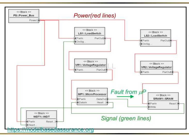
Architectural Models capture the structure and interconnection of the system and fault propagation SEAM/SysML: Functional Decomposition Model Example: Cubesat Experiment Board: Count Upsets in SRAM
