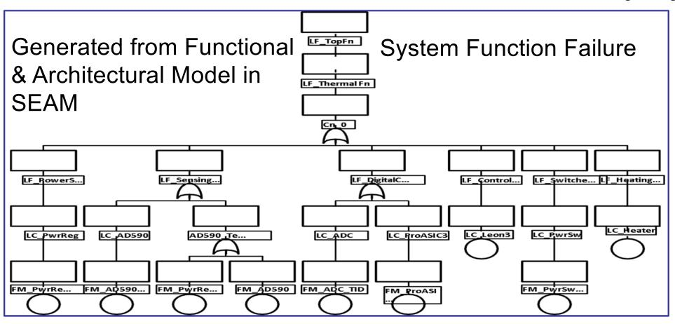
Component failure modes
