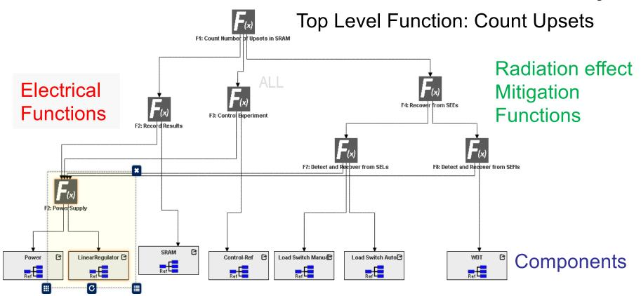
Functional Decomposition associates functions with component blocks <a href="https://modelbasedassurance.org">https://modelbasedassurance.org</a>
