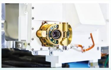
"The Scanning Habitable Environments with Raman & Luminescence for Organics & Chemicals (SHERLOC) is an arm-mounted, Deep UV (DUV) resonance Raman and fluorescence spectrometer utilizing a 248.6-nm DUV laser and <100 micron spot size. SHERLOC enables non-contact, spatially resolved, highly sensitivity detection and characterization of organics and minerals in the Martian surface and near subsurface."
