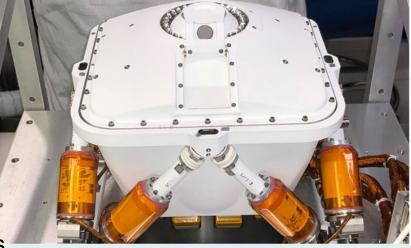
"The Planetary Instrument for X-ray Lithochemistry (PIXL) for the Mars-2020 rover is an X-ray fluorescence instrument that rapidly measures elemental chemistry at sub-millimeter scales by focusing an X-ray beam to a tiny spot on the target rock or soil and analyzing the induced X-ray fluorescence."
