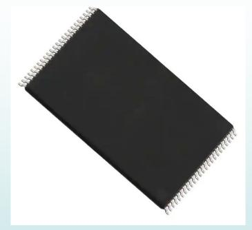
NAND flash stores data products which include the map data, algorithm outputs, including LVS results and all LCAM images
