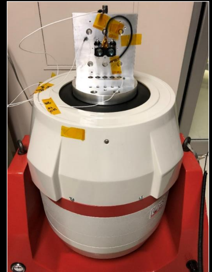
Garmin (candidate 2) on vibration shaker
