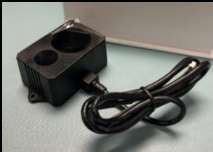
Mini LiDAR Candidate 3, which exhibited a clear performance anomaly post-vibration.
