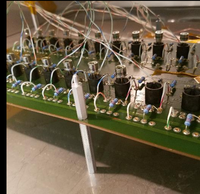
Detector samples shown in thermal chamber for burn-in testing
