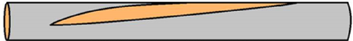
Bare strand (1 out of 19 showing bare copper region)
