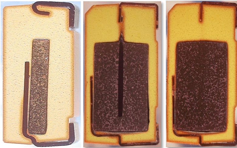
Parts with delamination
