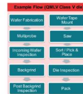
Figure 6. Texas Instruments example QML-V die flow.
