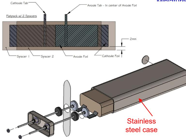
Hermetic Al capacitor overall construction schematic [5]
