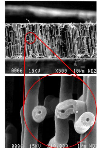
SEM images of anode foil dielectric on 400VDC rated Al electrolytic capacitor (surrounding Al removed). [4]
