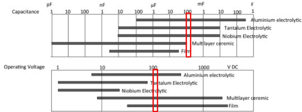
Ranges of capacitance and operating voltage of various capacitors.[1]
