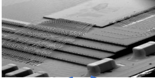
BGA with Internal Wire Bond
